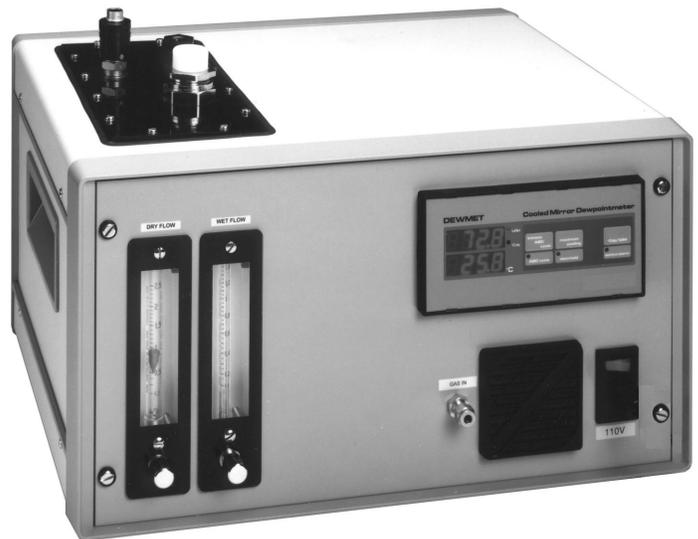
The Dewmet Hygrometer is ideally suited for the calibration of RH probes since it functions with great accuracy even at extreme RH levels. For example, the instrument operates from 2% RH to 99.5% RH with measurement accuracy of up to  $\pm 0.5\%$ .
