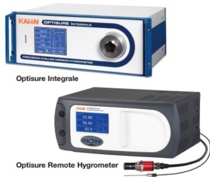
Figure 1: Optical (chilled mirror) hygrometers, like the Optisure pictured above, measure dewpoint by cooling a gas under test until dew or frost forms on a mirror. (Source: Kahn Instruments, Inc.)
