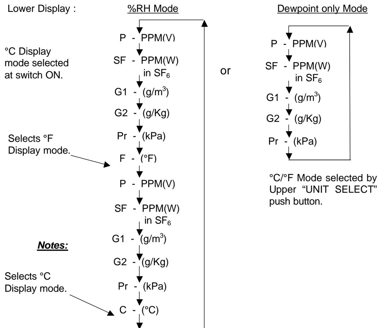
1. If a pressure transducer is not connected to the instrument, then by default, atmospheric pressure (101.3 kPa) is selected and displayed.
