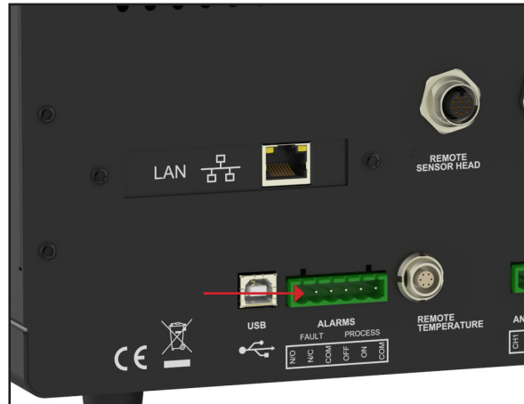
Figure 5 Alarm Output Connectors
