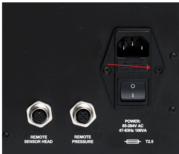
Figure 25 Power Supply Fuse Replacement
