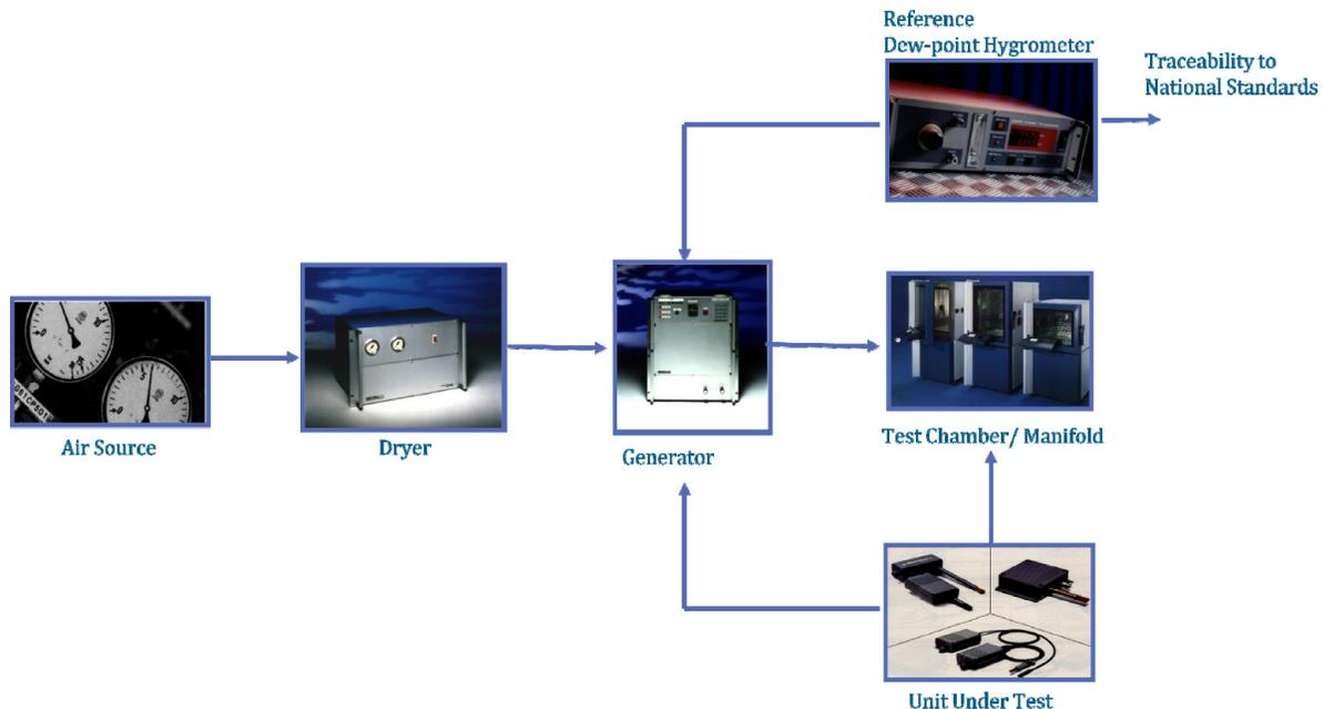
A dewpoint calibration system consists of the following components, which can appear in a number of different packages; a clean **compressed air supply** is required to feed a **pressure swing dryer**. This dryer provides a constant source of dry air, which provides the lowest calibration point, and also the base from which all other points are generated.
